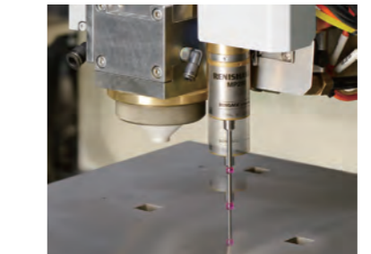
3D Level Adjust Correction function for workpiece upper surface
