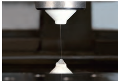
Jet feed unit for thin wire Wire feeding can be helped by water jet when using thin wire.
