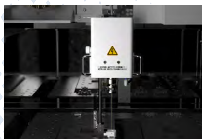
Start hole device (SHM2) including \Phi 1.0 pipe \Phi 0.3, \Phi 0.5, \Phi 0.8, \Phi 2.0, \Phi 3.0 selectable
