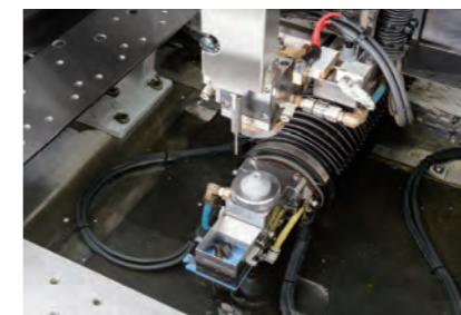
Core Catch Automatic device for core. This is used together with Core Stitch function. (Core Stitch function is necessary.)
